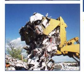
RyLind Multi-Purpose Buckets are designed to dig, scrape, clam, or bulldoze material. This multi-use bucket is for wheel loader, crawler loader or backhoe/loader applications. They work excellent in City applications handling everything from recycled asphalt and concrete to paper and plastic as well as construction and site prep work.
