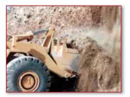
Rylind Rock Type Buckets are heavy duty buckets designed to handle rock, shale, slag, ore and other abrasive type materials.
