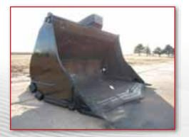
Rylind Spade Nose Mining Buckets are built entirely out of T1 and AR400 steel. The long lip, tapered side design for easier loading of blasted material. Available optional weld-on cast steel teeth, carbide impregnation, weld-on carbide plates, and shell liners are available in any configuration required. Roll Back cushions standard when bucket is cradled.
