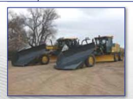
Rylind V-Type Snow Plows can be mounted on either Wheel Loaders or Motor Graders.
