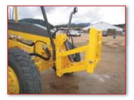
Rylind Front Mount Scarifiers mount to the head plate of a Motor Grader, and Rylind Quick Mount Scarifiers will attach to most major brands of Parallel Lift Groups.
