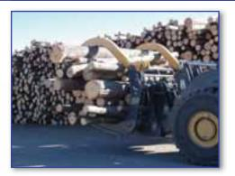
Rylind Mill Yard Forks come in Standard and High Capacity Designs, fast loading and large opening when picking up logs and brush from stacked piles. Double Top and Paddle Top Grapples Available.
