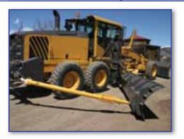
Rylind Hydraulic Snow Wings are completely Hydraulically operated no cables used. Moldboard, inboard, and outboard mechanical float system and spring loaded rear push-beam with shear-pin protection.
