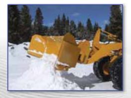
Rylind WAR Series Plows are designed with two angled out wings for heavy duty snow removal in parking lots, parking structures, city streets and airports.
