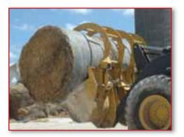
Rylind Grapple Buckets are designed for handling bulk materials like hay, brush, trash and other recycled materials. Weld-on grapple kits are available for your OEM bucket.
