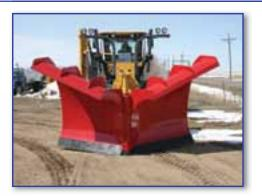
A true Folding V-Plow our MDPX Plow is built on our standard "MDP" frame, 42" tall at the center hinge pin and then extending to 70" tall on the outer snow flairs for faster snow clearing. Our MDPX Plow uses the same replacement parts as our MDP Series Snow Plows allowing for easy ordering and faster delivery. Dual flow control valves for cylinder protection from pressure spikes, 3/4x8 B/O Cutting Edges and 3" Center Hinge Pin with gusset reinforcement are some of the features.
