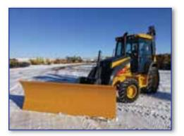
Rylind SRP Series Plows are a smaller ramp type plow with a more vertical 17° cutting angle and a rolled top snow shield built for smaller wheel loaders and loader backhoes.
