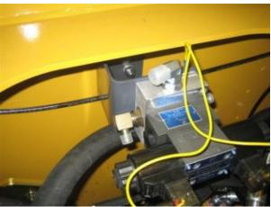
2. Run hoses from the coupler along the lift arms and down to valve using 1/4" blots and clips provided.
