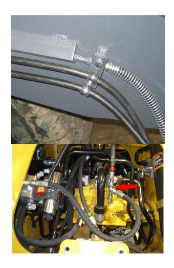
Run the provided return hose from port "T" on the valve to a convenient return source. (Return line, valve, tank, etc...)
