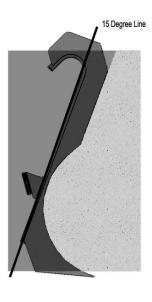
6. With the male coupler on the loader place mount the hooks on the coupler and lock the pins. Adjust the lower boom pin to match that found in step 1. Tilt the coupler 15 degrees forward. Be sure the hooks are square with the bottom of the bucket. Recheck height, centering, and square. (Image D)
